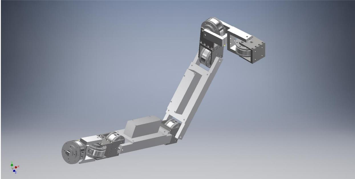
Lightweight aluminum construction, 250 lbs. repeatable load. Future conversion to plastic for lighter weight is possible. Four of these on a torso with hands and feet make a hydraulic humanoid.
